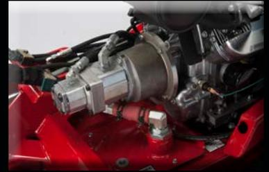
The engine is coupled to two piston pumps: a larger pump drives the cutter wheel and a smaller pump works the tilt and swing
